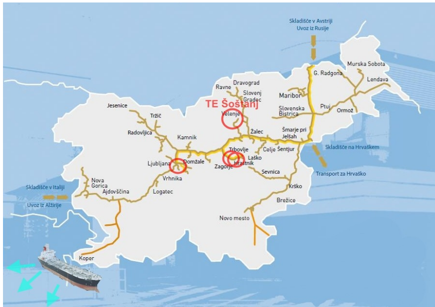
Figure 9: Gas transmission network and sources of CO 2 emissions suitable for the retrofitting the CCS technology
